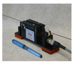
The detector uses two v-shaped flat ceramic guides to contact the wire. The ceramic guides are spring loaded. The guides move outward when a blister/ lump hits them.
